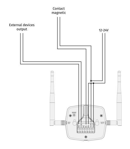
**Note** • If the device is connected with USB, to use the input, use an external 12/24V source.
